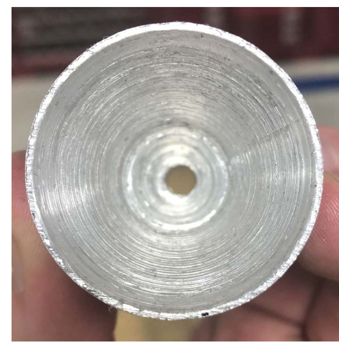
Machined ideal CON/DIV Nozzle insert (top view)
