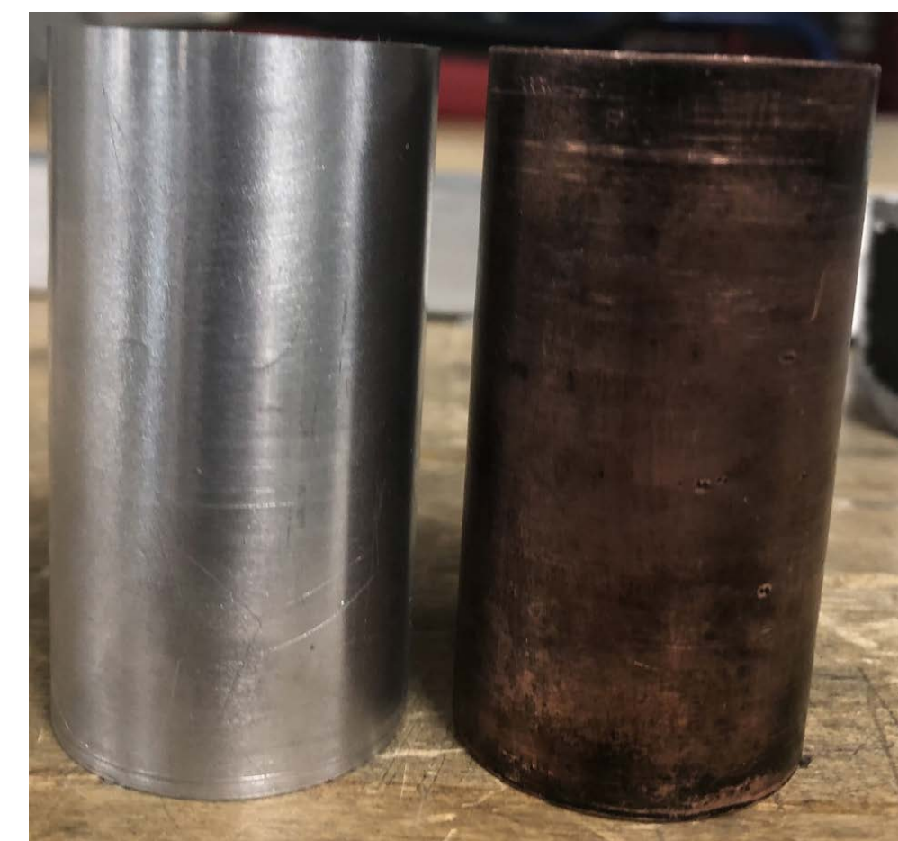
Machined ideal CON/DIV Nozzle insert (left, side view)
