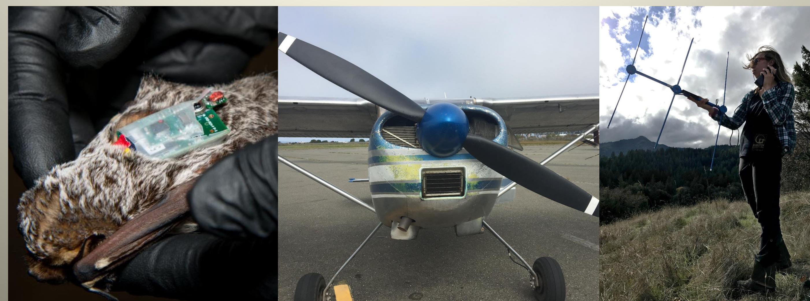
Figure 1: Miniature tags were deployed on wild hoary bats and later recovered using aerial and ground radio telemetry
